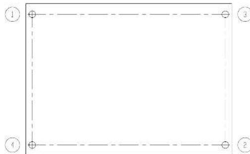
Figure 4 - 3 Bolts installation order (example)
