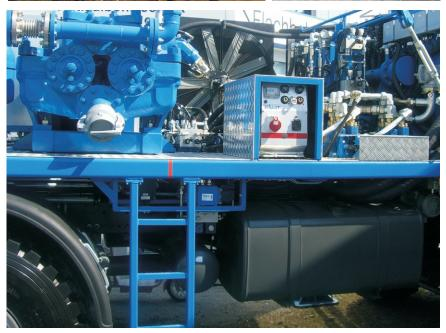
The hydraulic welder guarantees that high quality welding equipment always go along the work machine, even for continuous professional use.
